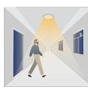
With insufficient daylight, the sensor turns light ON when motion gets detected.
