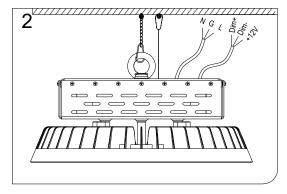
2. Connect chain and safety wire to the installation location, adjust the lamp high and level.
