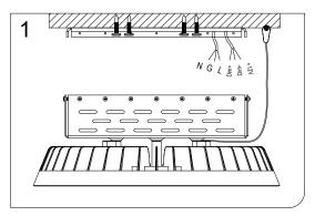
1. Remove the power box cover from the lamp, lock the power box cover to the ceiling with screws, and also lock the safety rope to the ceiling.
