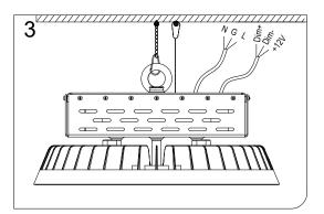
Connect the AC cable, L for the line, N for neutral, G for the ground. Adjust the light by positive and negative pole butt can.
