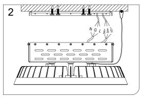
2. Connect the AC line and the adjustable light, and then lock the screws around the power box.
