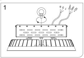
1. Take the fixture and hook ring out from cartoon box,tighten hook as arrow, fixed the hook screw.
