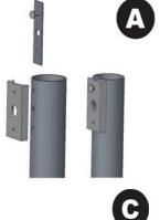
Step 1-Install the backplane and bracket adapter on the pole with top bolts, nuts and washers
