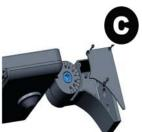
Step 3 - Hang the luminaire on top bolt (Figure C)
