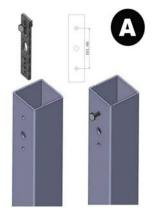
Step 1 - Install the back plate inside the pole with top bolt, nut and washer (Figure A)
