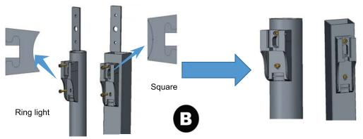
Step3: Fix the lamp body with the bracket installed to the bracket B of the pole and fix it with M4 screws. (Figu
