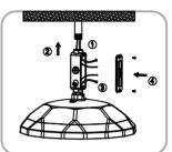
2.Thread the wire into the junction box, install the junction box on the pipe, wire according to the requirements, take protective measures, and lock the cover
