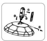
Remove the cover, thread the wire into the junction box, and tighten the terminal box and set screw
