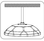
2. Rotate the lamp to the mounting pipe (rotate clockwise)
