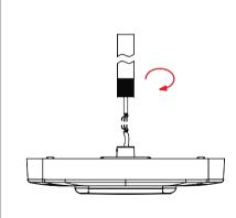
2. Rotating the 3/4 "NPT thread to make it fixed with lamp, and fix the NPT with supplied screw.
