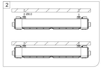
(2) a. Each side has two NPT 3/4" screw holes, which can be selected to open the cover on either side and connect the wire according to the L, N, G, L' mark on the terminals. b. Secure the fixture until it is tightened.
