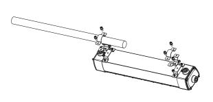
2. Put the pole provided to the top of your pole. Then tighten four set screws shown in the figure above.
