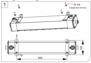
a. As shown in Fig. 1, drill four expansion bolt holes on the installation surface according to the size requirements, and install the expansion bolts.
