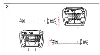
(2)a. Select any of the three 3/4 "NPT plugs as the interface for the cable input line. Select steel pipe or gland as needed, fill 16mm chemical filler to the wire tube, and then fix the wire tube to the lamp body (before installation must confirm whether there is a suitable gasket).
