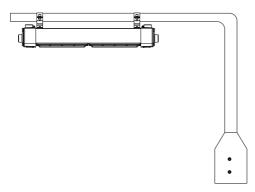
Properly connect wires and conduit. Each side has two NPT3/4" screw holes, which can be selected to open the cover on either side and connect the wire according to the L, N, G, L' mark on the terminals.
