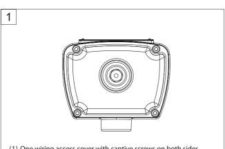
(1) One wiring access cover with captive screws on both sides. Open the cover with an Allen Key.
