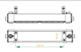
1. Fix the lamp to the pole provided by mounting bracket welded at the back of lamp. Tighten the screws on the mounting bracket .
