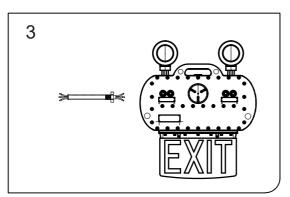
3. Install pipe to 3/4" NPT entry and fix16mm (0.63inch) Chico A. Then connect the AC cable: black cable joins to L,white cable joins to N, green cable joins to grounding.
