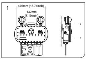
1. Drill four holes as fig. 1, the distance as per 476mm (18.74inch) and 132mm (5.19inch).
