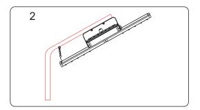
2. Fix the pendant chain and hook the fixture. Insert 2x Ø15 fixing screws and weld them on the pole bracket with the fixture.
