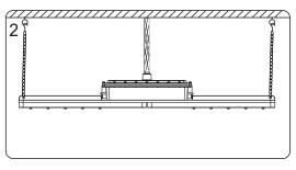
2. Fix the hanging chain to light fixture. Wire the cable through the metal conduit and then connect it with the power.
