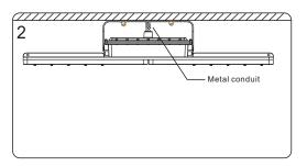
2. Install the fixture to the expanded screws, and tighten the nuts. (Metal conduit needs to be applied here)
