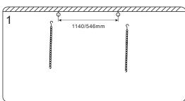
1. Drill 2x hole for hanging ring(1140mm for 4FT fixture or 546mm for 2FT fixture), and fixing them.
