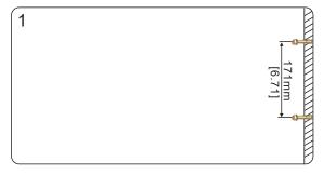
1. Drill 2x Ø15 hole for expanded screws, and fix them to the wall. (Horizontal distance: 171mm)
