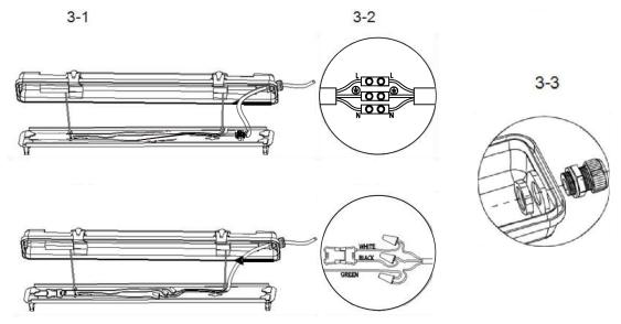
4. Fix the reflector by bracket, put the tube into the lamp holder, lock the base and diffuser by clips.
