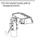
of lamp pole is Ø60, lamp adjustable angle is 0-90°.
