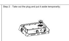
Step3: Take out the plug and put it aside temporarily; set power and CCT switch to the corresponding position
