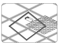
c) Take off knock-out one the other side, connect all wires with the AC input properly according to the labels on wires.
