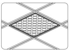
f) Put the driver cover back and well installed. Driver should not be mounted in or near a fan air outletor or other HVAC system conponents.
