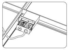
d) Remove the plasterboard and install the fram light in the T-bar.
