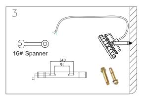
3. Drill 2x hole as Fig.2, the distance can be  $91^{\sim}140$ mm, fixing  $\varnothing$ 10 expansion screws and bracket on ceiling.
