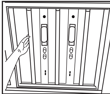
2. Remove the fluorescent Tubes & ballast
