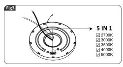
4 Connect supply wires to wires on fixture/ bracket with wire nuts. Attach white to white, black to black, and copper wire to green wire as grounding connection, Connect the safety rope to the installation plate for a secure fit. see Fig4.
