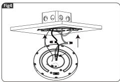
**5.** Arrange the wires into the J-Box.
